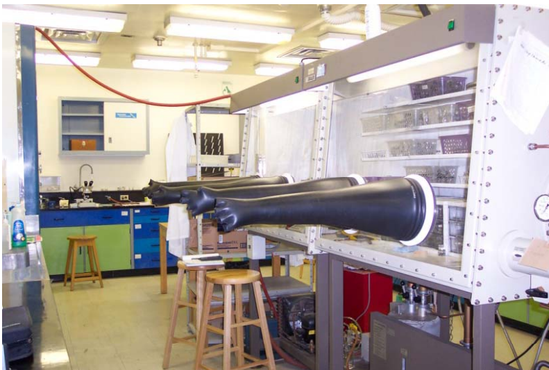
Working Under Inert Gas Atmosphere
