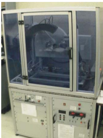
Collection Of Powder Diffraction Data For Phase Analysis
