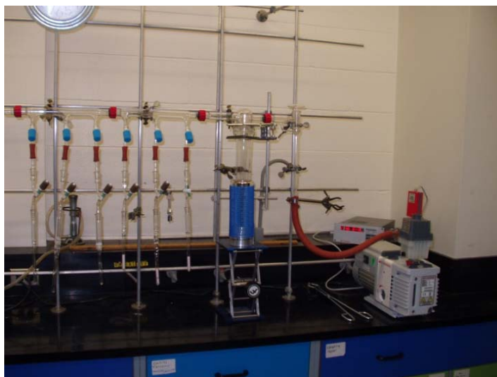
Evacuating Of Sample Vessels
