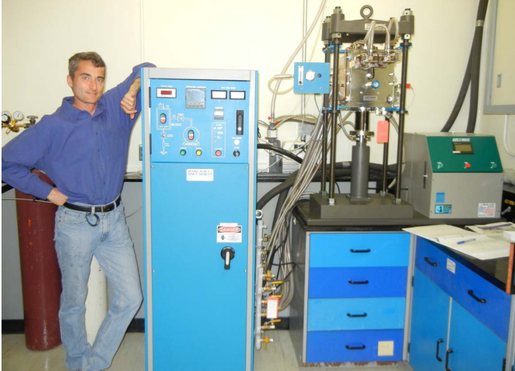
Controlled Pressing With 30 Tons Below 1600°C For Hours
