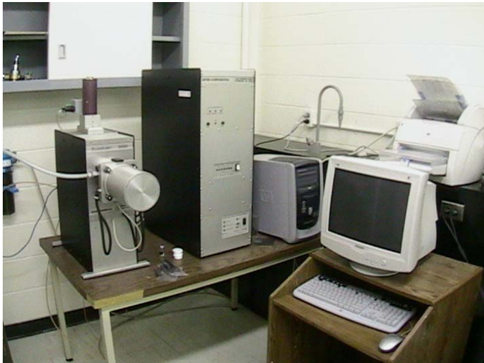
Determining Thermal Conductivity Between 25°C And 1000°C
